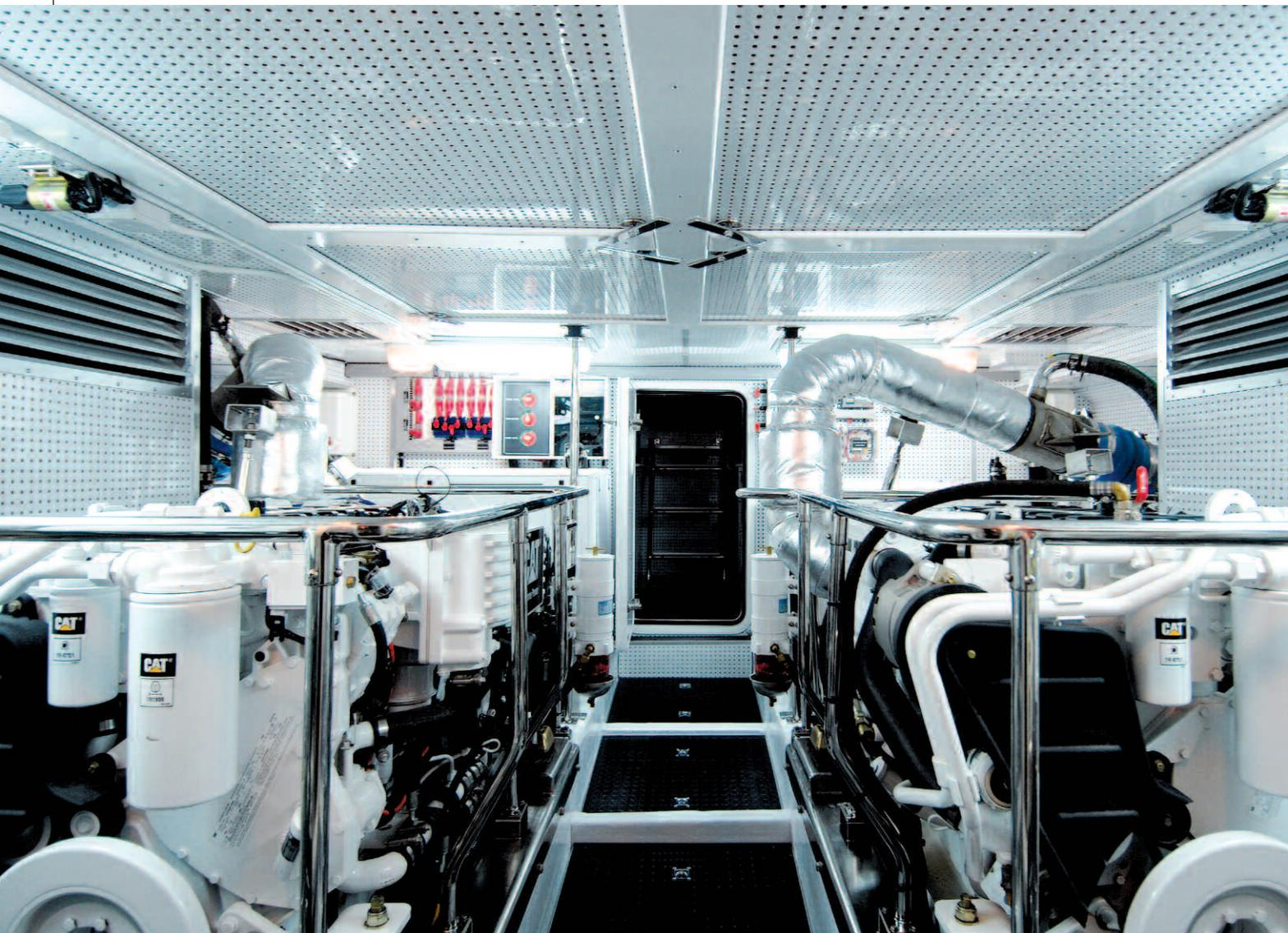
The OR 63's well-lit engine room is laid out for easy access during routine maintenance and is thoroughly insulated to reduce noise.
