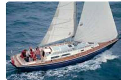
In keeping with her traditional hull, the 36 has a simple twin-spreader masthead rig with forward and after lower shrouds. Lead ballast encapsulated in a fiberglass molding that's part of the hull eliminates keel-bolt problems and leaks.
