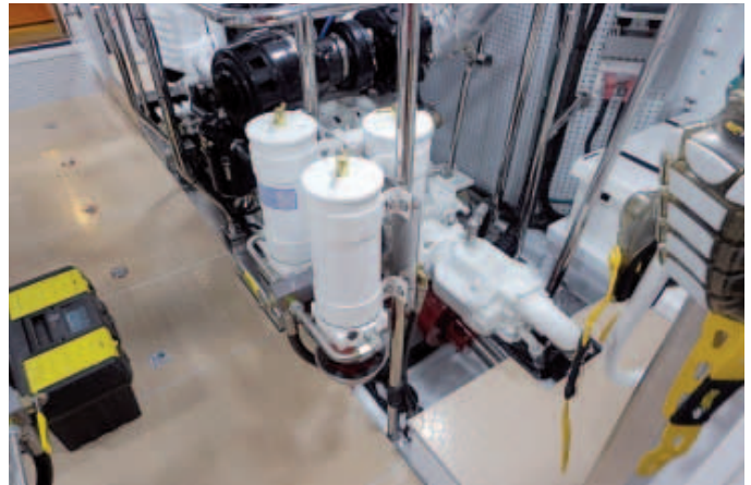
Above left: The captain's cabin is luxuriously appointed with double berth and ensuite head. Top right: Tidy and clearly labeled fuel manifolds make transfers easy and intuitive using the combined pump and fuel polisher. Above right: Nonskid walkways, solid safety rails, and an easily accessible trio of fuel filters mark the engine room.
