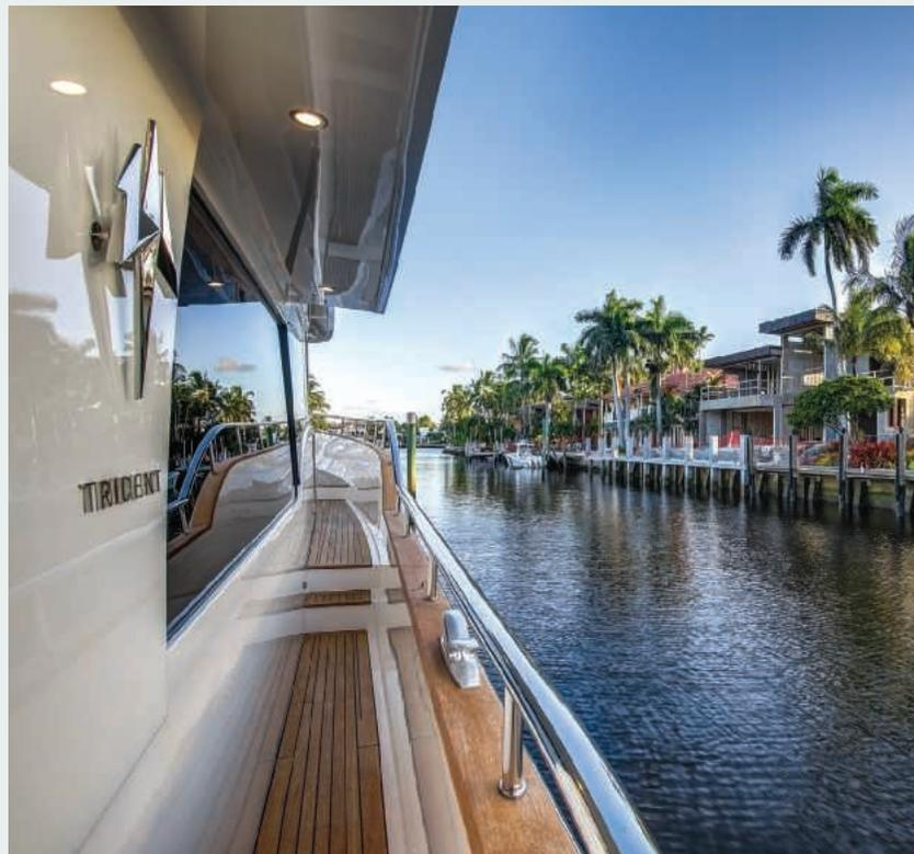
The 620 Trident's side decks are built for safe ocean passages, with high bulwarks and stainless-steel handrails.
