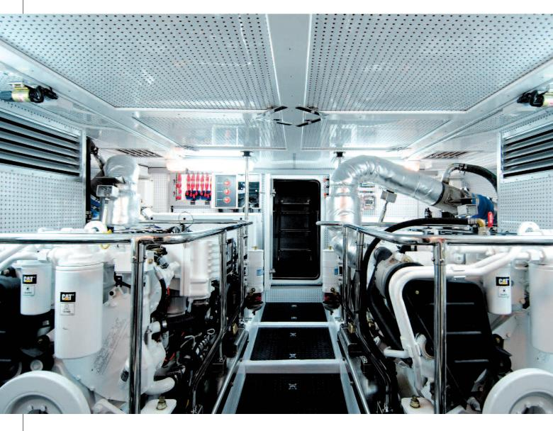
The OR 63's well-lit engine room is laid out for easy access during routine maintenance and is thoroughly insulated to reduce noise.
