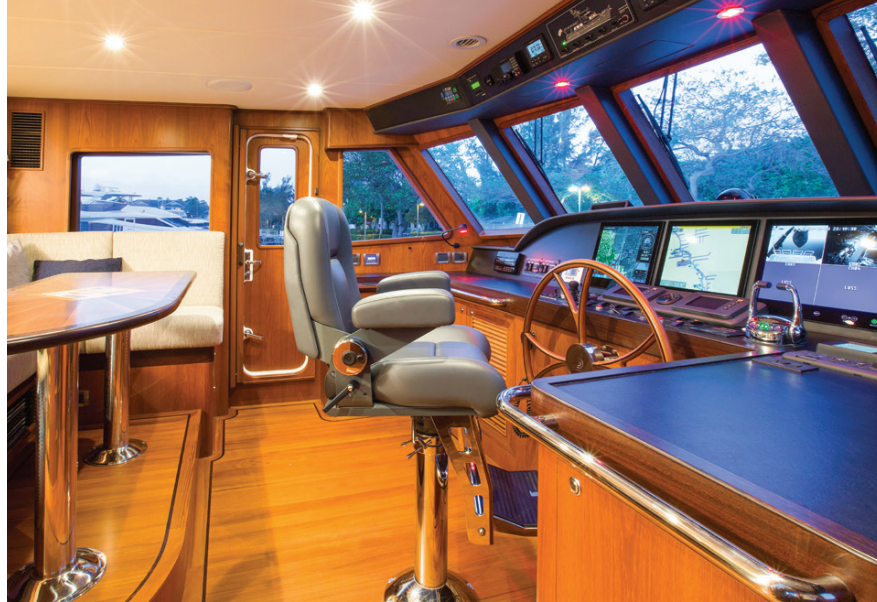
The interior helm has everything a captain needs to drive and monitor the yacht, but the dash is shallow and low profile, so it doesn't intrude on living space.
